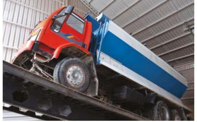
They are hydraulic mechanisms built for trucks to unload their goods. Side or back covers may be used for unloading.
