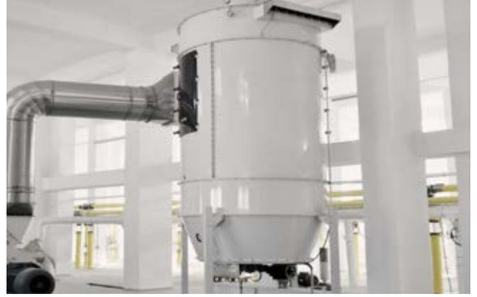
Jet Filter is applied with advantage for achieving efficient separation of dust particles from a dust-and-air mixture Round filter body firstly purifies the mixture with the cyclone system so that dust particles are held in bags.
