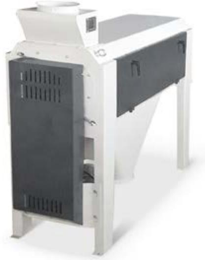
The product is conveyed to the sifter. The special arrangement blades of the rotor throw the product to the cylindrical screen. Big undesirable materials are conveyed to the discharging unit from inside.
