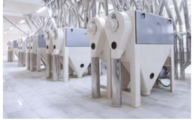
It is used for separating the flour particles which stick on the bran. It helps to increase the performance of the system.
