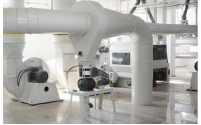
It is used after air channels and before the filter or central dust cyclone in the cleaning section. It prevents foreign heavy materials in the air. Thus it provides the system run efficiently. Also, it protects the filter bags.
