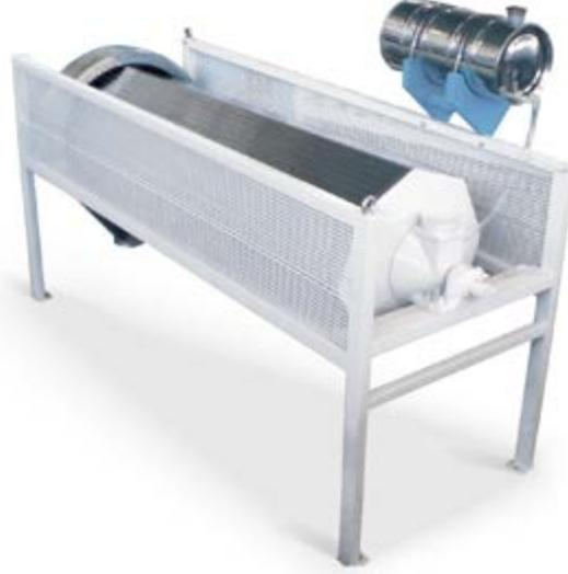
Oiling machines are used after finishing the processing of rice and just before the storage to make the rice bright by using 0,35% oil . beside making the rice brighter it also provides longer shelf life for the rice.
