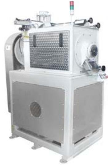
Pneumatic polish machines carry out the process of polishing the surface of the rice with the files in the paddy processing plants. Also increasing the quality of the rice, with polishing ,whose quality is low.
