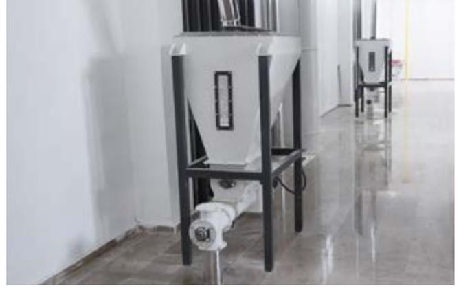
It is used in the filter outlet and under the ofal depots. It is used to get back and add the product that is leftover in the filter to the system. Its design is plain.
