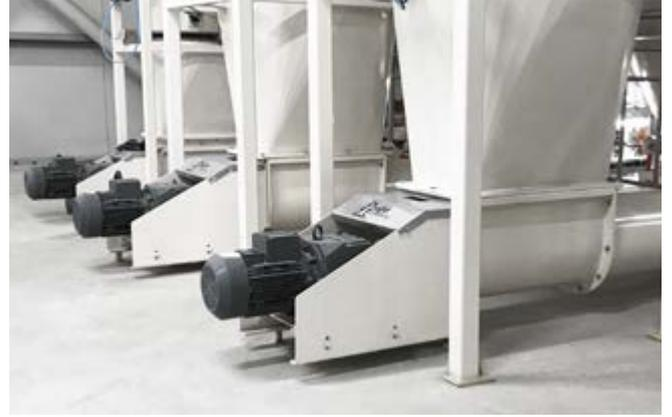
The tube screw conveyor is used for the transportation of all floured thin and middle ground products vertically and inclined to the screw conveyor. Reductor motor transports its power through coupling connected to the motor, to conveyor shaft. With the help of the spiral of the conveyor shaft, the product flows through inlet bunker to outlet bunker, and then it is taken to screw conveyor or elevator.
