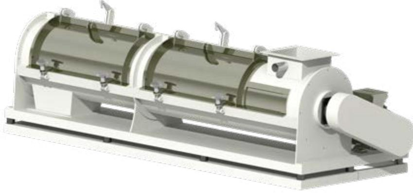
It is designed for homogeneous mixing of fluid sweetener to product additives in feed mill plants.
