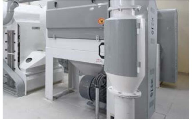
It is used to separate iron pieces from products in grain and pulses plants. Because of natural magnet power, it doesn't need any energy consumption
