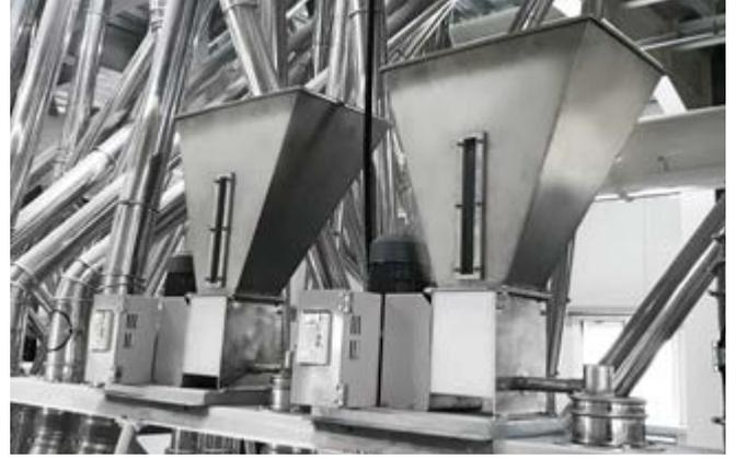
It supplies to mix the requested amount of vitamin into the ground product and to be mixed into the system. It has the speed control advice that helps to work the system easily and properly. It dosages the improver into the flour. There is a special mixer in the bin.
