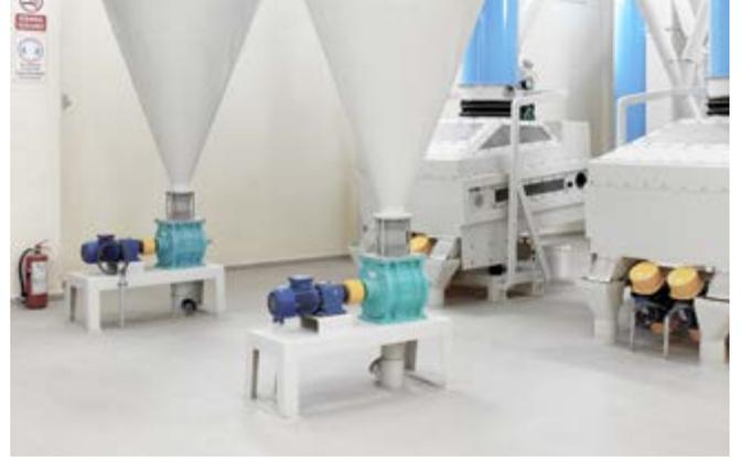
It is used in the aspiration system of plants. It generally collects the dust of grain, separates dust from the air, located in the aspiration system of cleaning machines. The specks of dust which are taken by aspiration get separated from the air thanks to the cyclone.
