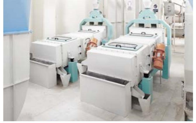
It is used for separating foreign materials from the grains. It has an adjustable angle of dip and vibration system. Low energy consumption, high-performance, high throughput, easy maintenance, long life. Fast and easy sifter change and easy cleaning. Silent running.
