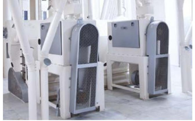
It is used at the first and second cleaning sections in the flour and semolina mills. It has an excellent scouring effect. It is applied in grain milling in both the first and second cleaning stages for the intensive surface treatment of numerous different grain varieties. It efficiently removes impurities such as dust, sand, clods of soil, etc. that adhere to the grain, thus providing ideal preparation for grinding.
