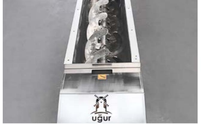
Palette conveyor is used to transporting dampened wheat horizontally. Palette conveyor is used to carrying dampened wheat without breaking it.
