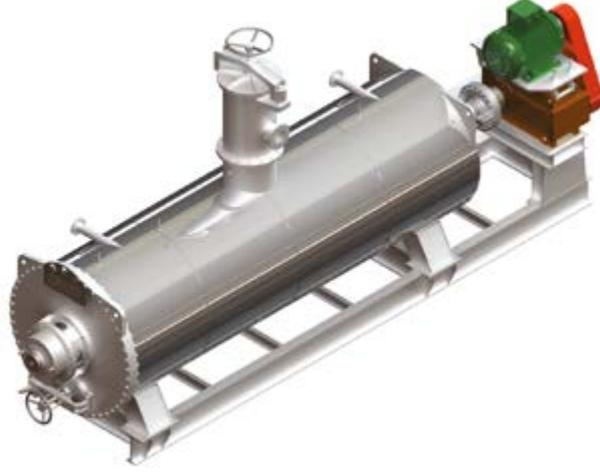
This unit is used producing feed additives by cooking of poultry feces.
