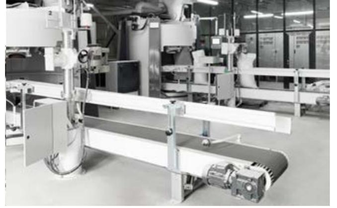
It transports the bagged product from one place to another. Its transportation system works by combined conveyor band.
