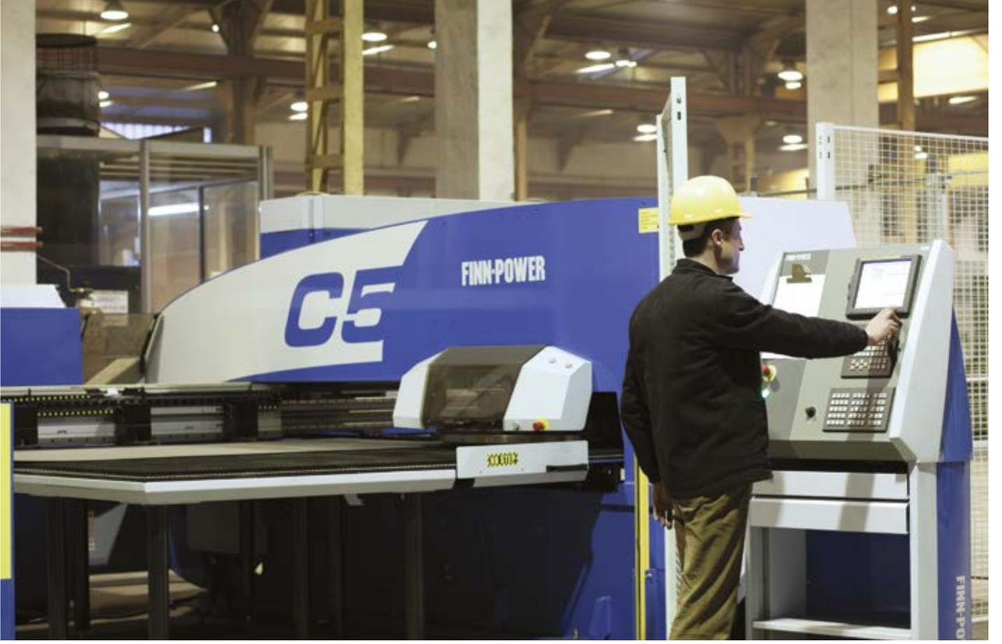
Applying the metal plate punching and cutting machine.
