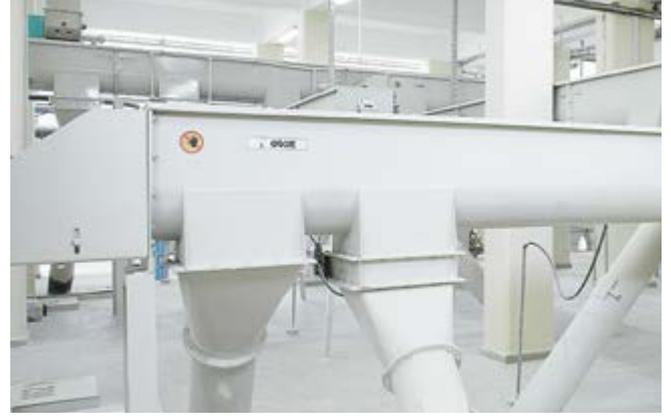
Its usage area is the discharging system of the screw conveyor. It is preferred to use in automation system plants.
