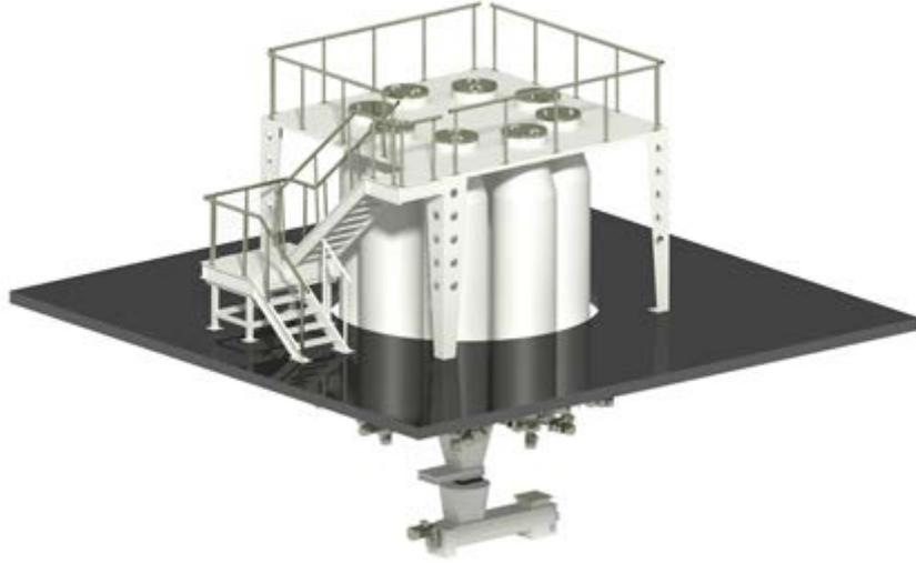
Microdosing systems make a sensitive weighing which is required for the addition of micro elements to feed while manufacturing.
