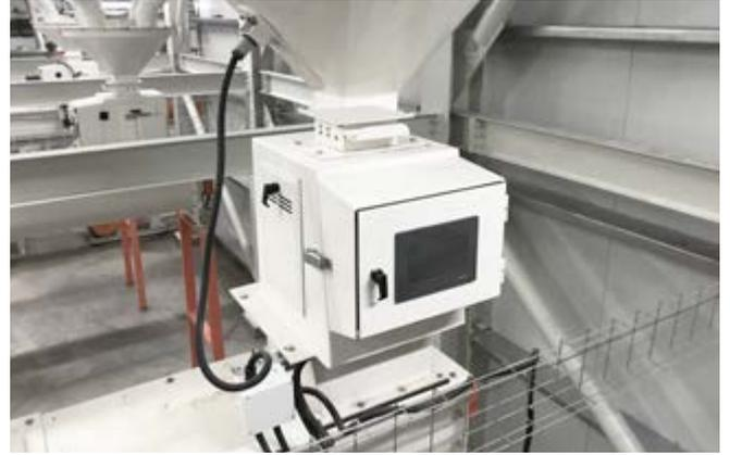
This machine is used for the capacity adjustment and the mixing of different kinds of grain in requested rates automatically by the operator panel before the grinding of grain.
