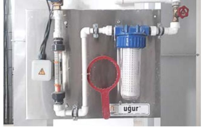
It is used to dose water for wheat dampening. When the sensor receives the wheat, the valve which provides the water control in the system is opened and closed automatically. Adjustable water dosing and sight glass level indicator. Before adding water to the system, water passes through the filter.
