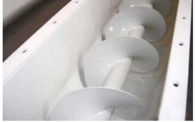
The screw conveyor is used to transport grain and finished products horizontally. The power of the machine should be adjusted well and according to the capacity to make it work constantly and effectively.
