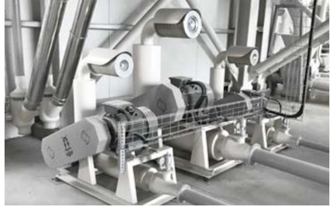
It is used for the horizontal or vertical transfer of all kinds of grain and pulses. Also, it is used to clean the filter bags. Direct-coupled and belt pulleys operation is both available.
