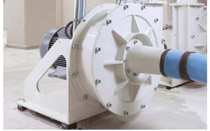
Insect larvae pass through silk holes with flour grow and become insects in a short time especially in hot environments. Entoleter prevents growing and increasing of insects by means of cleaving larvae in the flour by high speed gyring. It is manufactured with different capacities as 2-5-10-22 tons/hour. Installation can be before the bagging or the inlet of flour silos.
