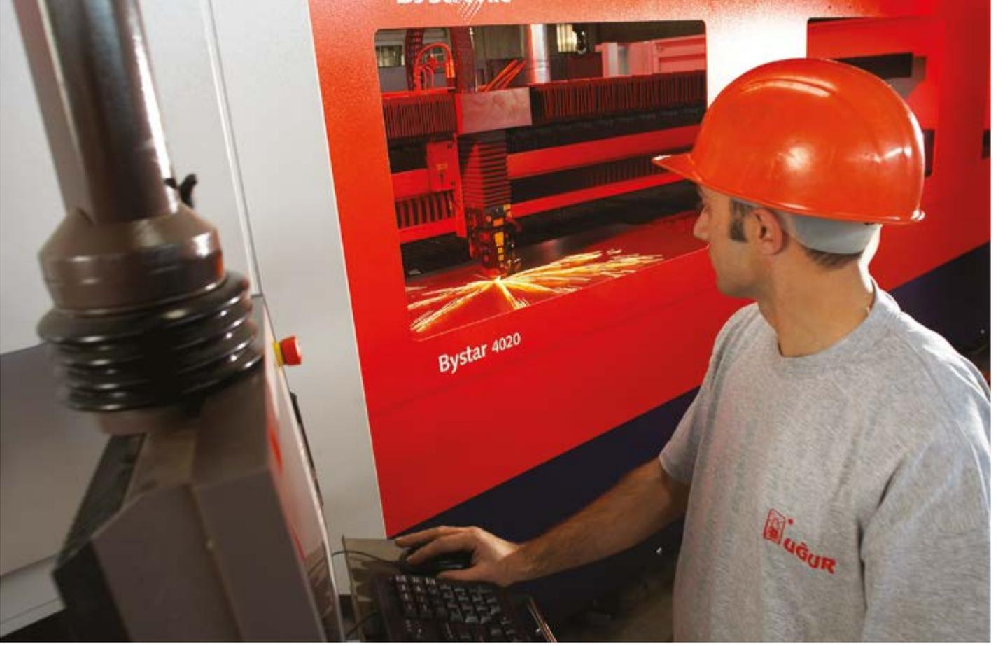
CNC cutting is used for cutting of hard metals. Particularly it is used to make cutting in demanded scale and dimension in steel construction projects. Due to its quick cutting it is time saving.
