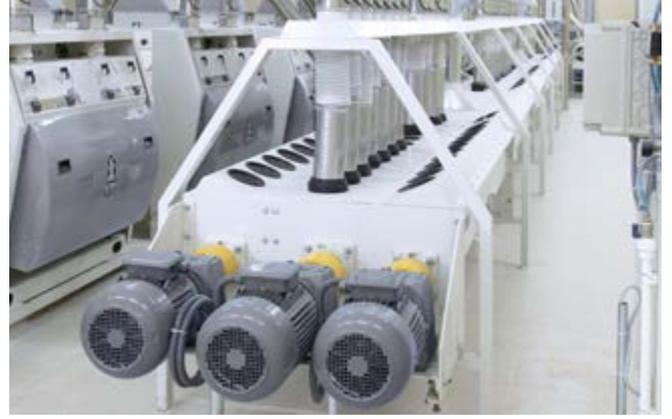
The screw conveyor is used to transport finished products horizontally. It is used to transport finished products from different passages to the intended place (silo or packing place). It has a very efficient using and it can easily replace thanks to its flap valves. It presents efficient using in flour, semolina – maize milling plants. It has a "U" shaped body.
