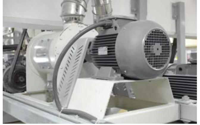
The Drum Detacher is used for the separation semolina and brand pieces which are stuck on to each other in the roller mills. Soft separation operation does not affect the product
