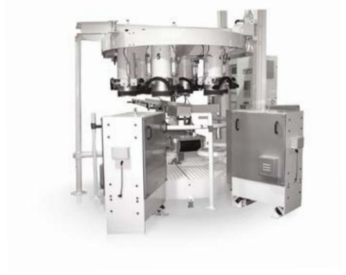
High capacity packing machine makes sensitive and high extraction packing. This is one of the most important machines of high capacity mills. Important saving from the labor. It reaches a maximum capacity of 40 tons/hour.
