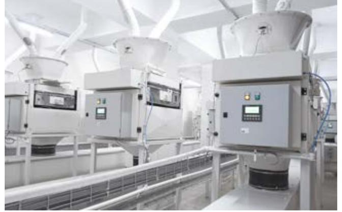
Permanent and precise measurement for the wheat that passes through.
