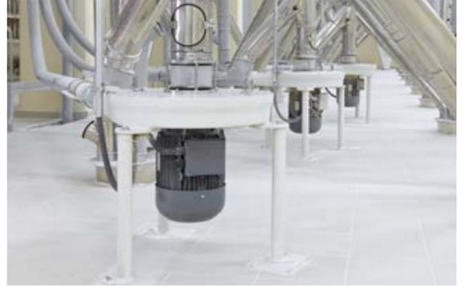
It is used for the sections that have so much to increase the efficiency As an assistant of the roller mills. It completely manufactures metal construction. It's available to use in the bottom outlet of roller mill or the section of pneumatic steel pipe. It can install on the floor or hang from the ceiling. The impact wheel is fitted directly onto the motor shaft. Flanged type motor (5,5 kW-7,5 kW) is used according to capacity.
