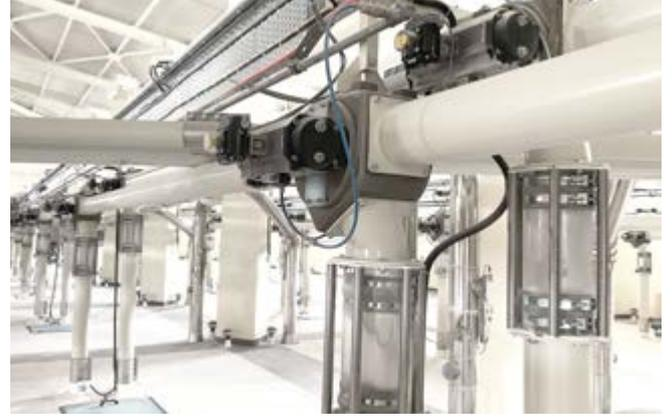
Especially in the food industry, and also in plastic, medicine, and chemistry industries, this machine is used to send the dust particles from one location to another location. It is manufactured by 27mm-168mm diameters steel pipes. It's preferred in automation system plants.
