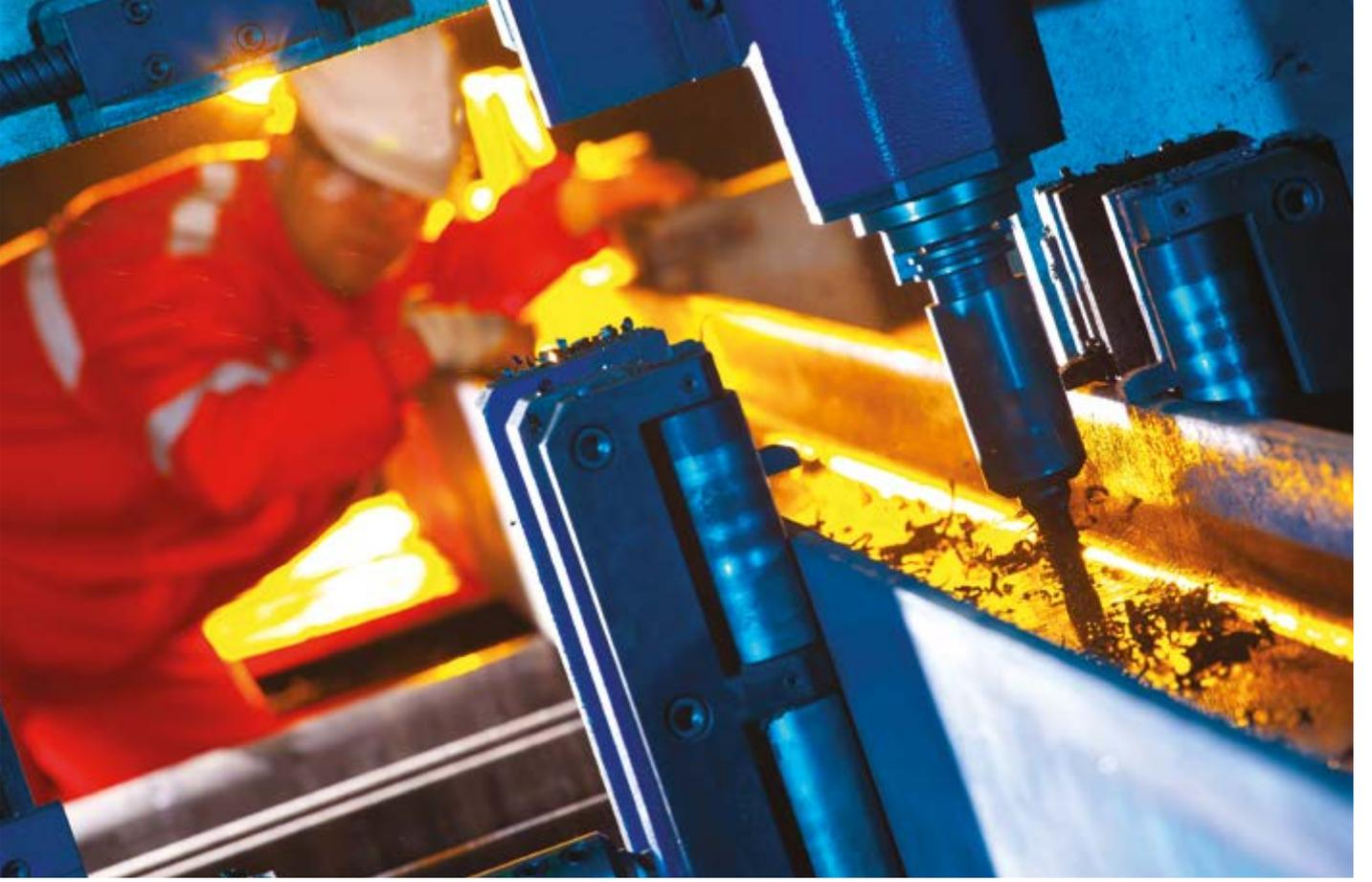
His machine provides cutting holes in desired dimensions and numbers in steel materials.
