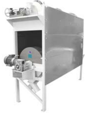
Broken trieur is used for separating the broken rice from the processed rice in the plant. With the press feature in the sieve system; via length difference it separates the broken rice from the rice. The machine is produced as 2 storey.
