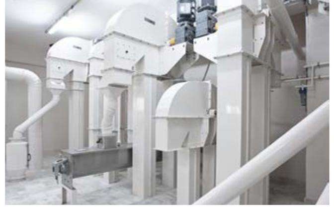
The bucket elevator with buckets hold on belts is used for the transportation of grain or powdered product from downstairs to upstairs. They are produced according to their capacity.
