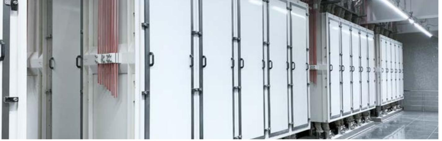
The Square Plansifter is a very important machine for the process of flour production. It is used to sift and classify ground grain that comes from the roller mill. The sifting process of arranging is according to the milling diagram. The Plansifter consists of;
