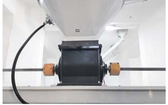
This machine is used for the capacity adjustment and the mixing of different kinds of grain in requested rates manually by the operator panel before the grinding of grain.
