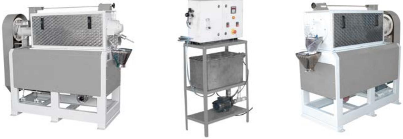
Rice, through a sanding process on Horizontal Whitening Stone machine for the receipt of rice bran. With this sanding process, surface of rice becomes nicked. In the following process the nicks fills with bran. These bran remains, with the effect of fatty acids in them are exposed to oxidation in time. With the effect of this oxidation, rice will become smelly and sour.
