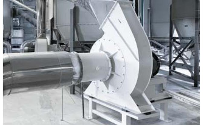
It is the system which sucks the broken products coming from the Roller mill. It has high production, a low energy consumption, multi-purposed and runs very quiet.
