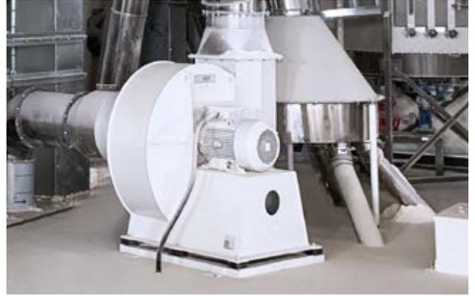
Low-Pressure aspirators are used in industrial companies, food sector, heating and aeration plants and also in the casting industry. The types of aspirators that are chosen according to the value of flow and pressure are used by different motor powers. They are especially used in the food sector to help cleaning the grain and the classification of the product by air.
