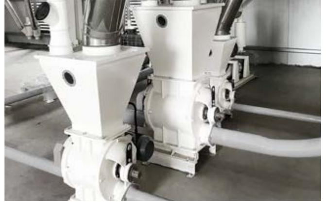
It is used to feed the product regularly and without leaking out into pneumatic conveying pipes at the pneumatic conveying systems.
