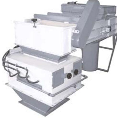
Pellet oil coating unit is designed to coat cooled pellet passing on band by spraying of oil, liquid enzyme and methionine.
