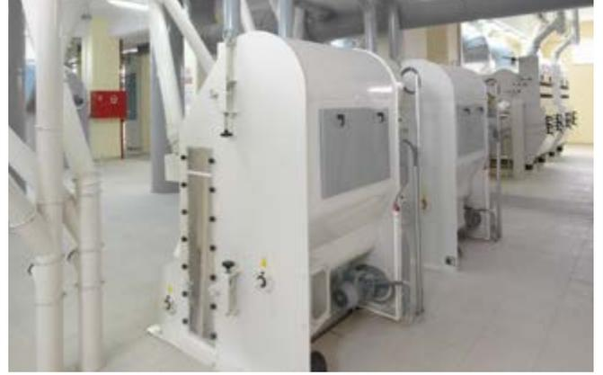
This machine is used for the separation of low-density materials, from heavy density grains such as wheat, rye, barley, oat and maize in an aspiration channel.
